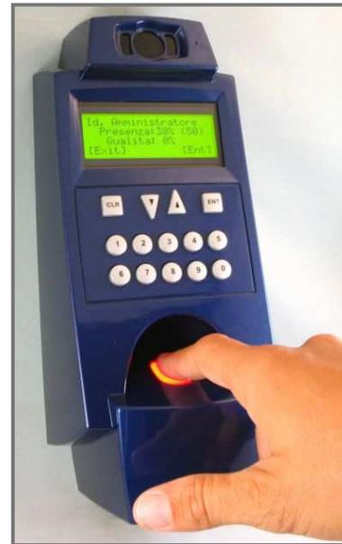
FxLock is a professional biometric terminal for fingerprint-based access control and time&attendance applications.
